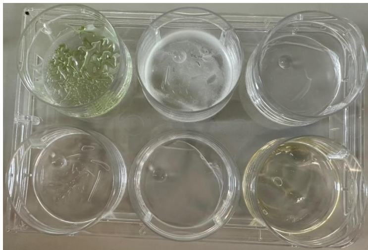
Figure 1: Water droplets on manufactured SLIPS systems. Counterclockwise from top right to left: perfluorodecalin, coconut oil, clove oil, olive oil, Novec 7500 (not analysed) and silicone oil
